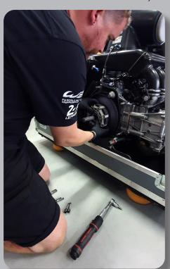
valuable points. Gulf Racing has been using Norbar torque products since 2017, and have a high level of confidence in our tools, and are always content using them for critical bolted assemblies. In this case study we look at the installation of a performance clutch assembly, something which if incorrectly installed can significantly impair the car's on track performance, both during practice, qualifying and race sessions.
